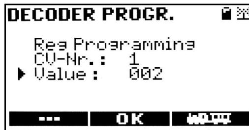
Register programming was the first method of CV programming. This old method is still supported in order to be compatible to outdated central stations and programming units. The CV value is to be entered into an intermediate variable. The decoder thereafter does the real programming. The input into register 5 and 6 is accomplished in this menu window. The CV 1 to 4 are entered directly; all other CVs with higher numbers are programmed indirectly (by register programming)
