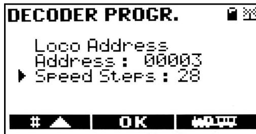
This is the menu window for brief locomotive programming. The number of addresses selectable is 1-10239. The DiMAX Navigator computes automatically the appropriate values for CV's 1, 17, and 18. In addition, speed steps can be set to 14 or 28.
